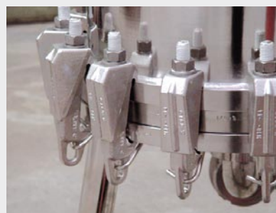
Closing mechanism with swing bolts.
