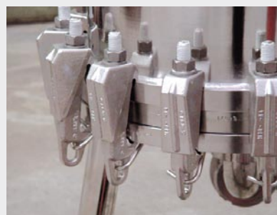
Closing mechanism with swing bolts.
